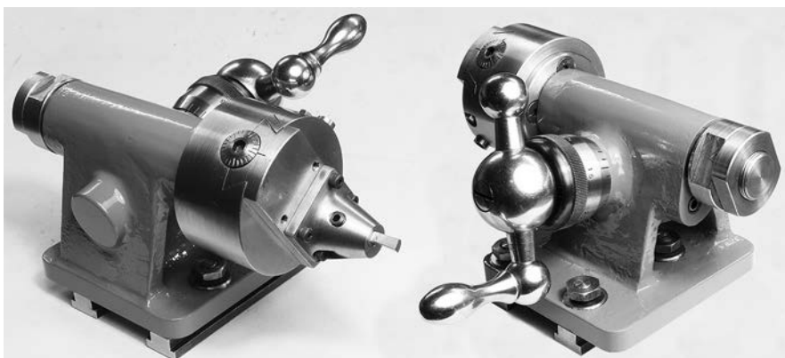
Figure 9 The completed turning attachment. The size B2 ball clamping handle has yet to be fitted to the sliding block
