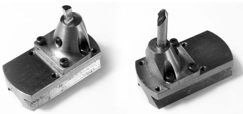
Figure 7 The tool holder, and (right) showing a broken BS2 centre drill from which the tool bit can be ground
