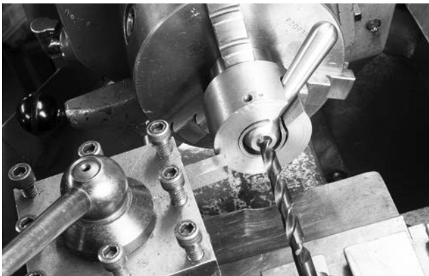
Figure 13 Making a one-ball lever handle
